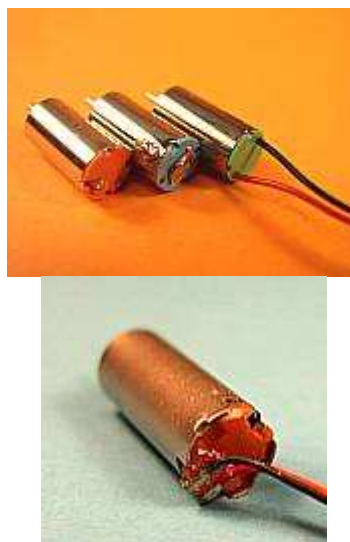
Connection methods left to right: side-bell contact, center-bell contact, wire connections. The picture on the right shows the distinctive connections for the surplus 6.1mm brown bell pager.
